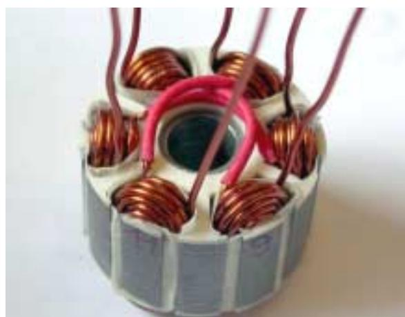
When the stator bushing is finally installed, take care, that one of the threaded holes of the mounting flange points exactly to tooth 11 of the stator. This allows an optimized wiring of the controller terminals through the front shield.
