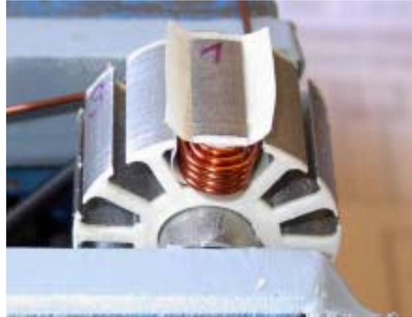
Before the second or third last turn justify the excess length of the fishpaper at the two unwound neighbour teeth. The two internal projections are shortened to 3-4mm and slid under the exterior. This groove cover can additionally be sealed with superglue - surplus adhesive has to be removed immediately.
