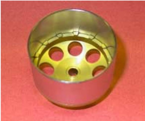
First, the parts which are to be glued must be prepared. Roughen the inside surface of the inference ring with fine sandpaper and degrease it with acetone or alcohol. Do the same for the flange of the driver plate which contacts the inference ring. Spread the flange thin with UHU-Plus (fill up groove), but keep the magnet alignment teeth free of glue. Slide the driver plate slowly into the inference ring as far as possible.
