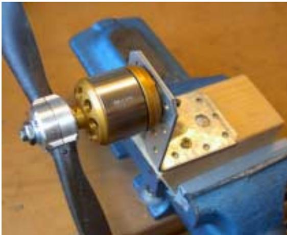
If that works you can try to use the motor loaded, which means with attached propeller. Check and make sure you have enough room first – the propeller shouldn't be able to hit anything. **Always** start the motor standing **behind** it – if a propeller tackles it can only fly to the front or the side (if the propeller tears to the front).
