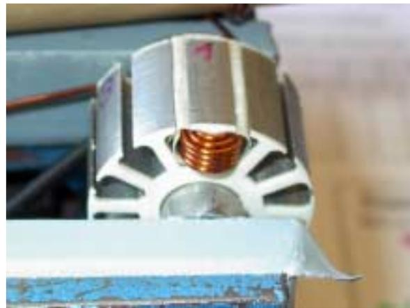
Take the stator block out of the vice and unwind the loose end from the stator bushing. Check the position of the protection tube on the wire and correct if required.
