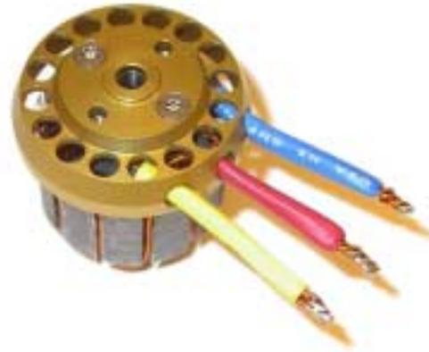
Strip all wire ends carefully for about 10mm with a sharp knife (remove **all** isolation !) and apply tin to the singular wires. Twist the ends as shown and solder the wires together. Install the front shield and fix it with 2 screws included in the kit). This step finishes stator assembly, which is most of the overall work.
