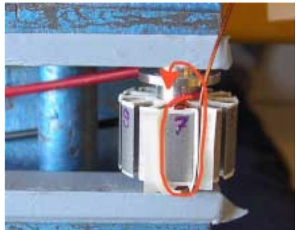
Wrap the wire around the stator bushing to the second tooth (tooth 7) and thread it into the slot. Clasp the stator back into the vice with tooth 7 pointing up and wind the second tooth in the same rotational direction.
